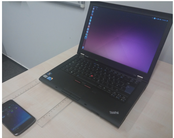
Fig. 3. Demonstration of the working environment. Smartphone is silently receiving EM-signal from the laptop at the distance of 12cm.
